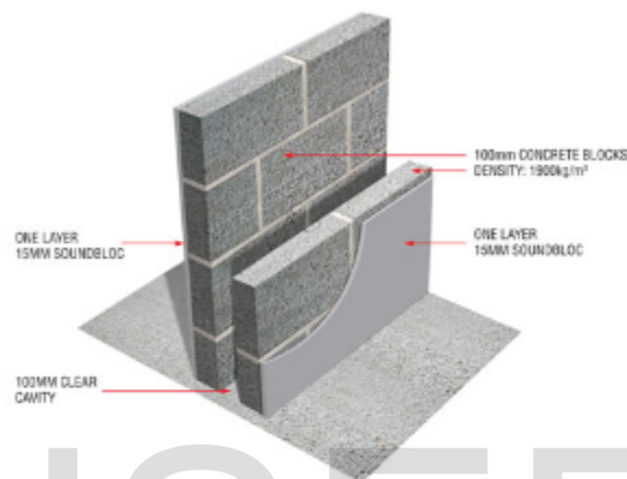
Fig 50 : Foam Concrete Cavity Wall
